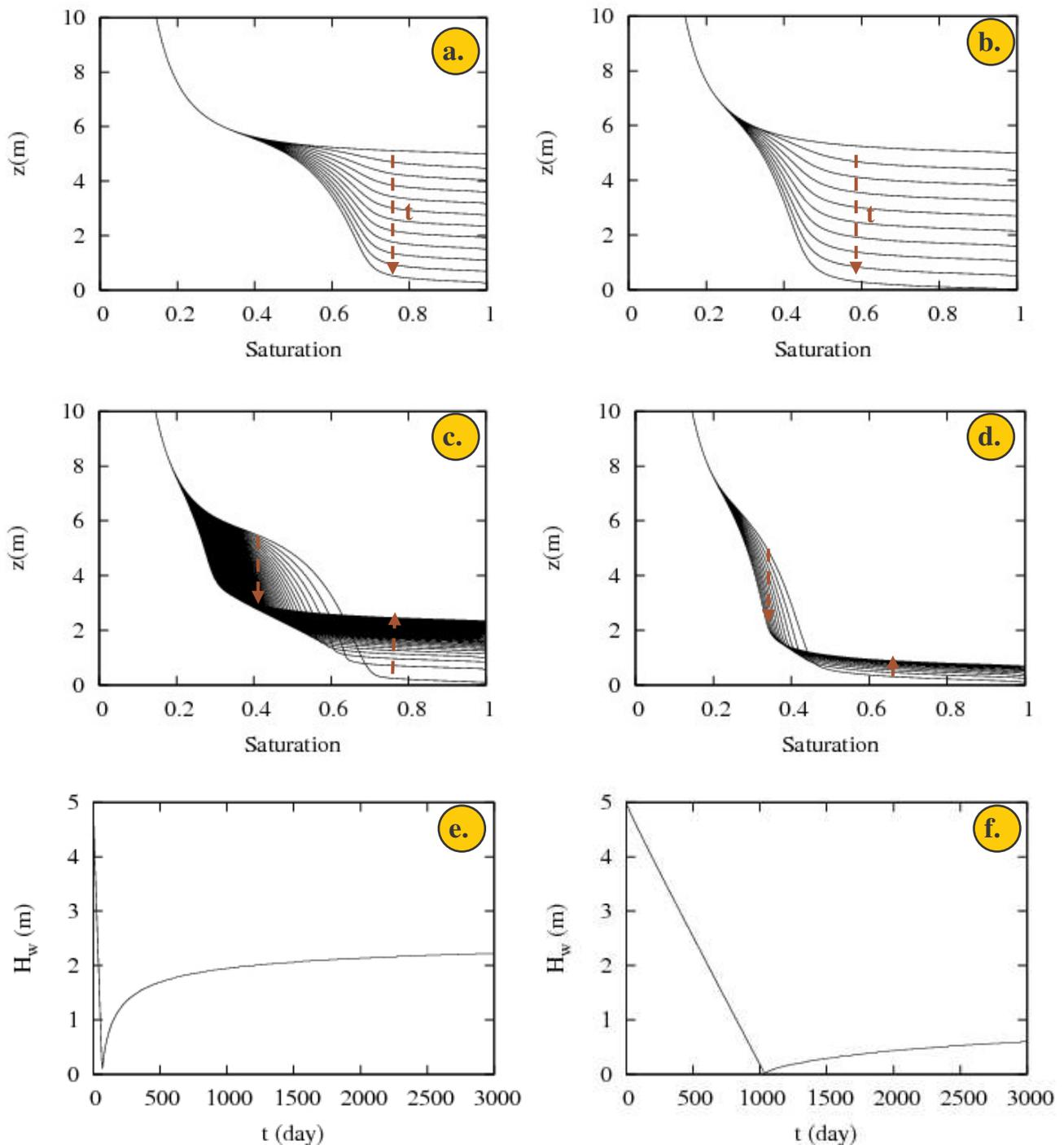
Figure 5. Influence of the pumping flux on the moisture distribution [High pumping flux (a, c, e) - Low pumping flux (b, d, f)] [Pumping phase (a, b) - Relaxation phase (c, d) - Water table level versus time (e, f)].
