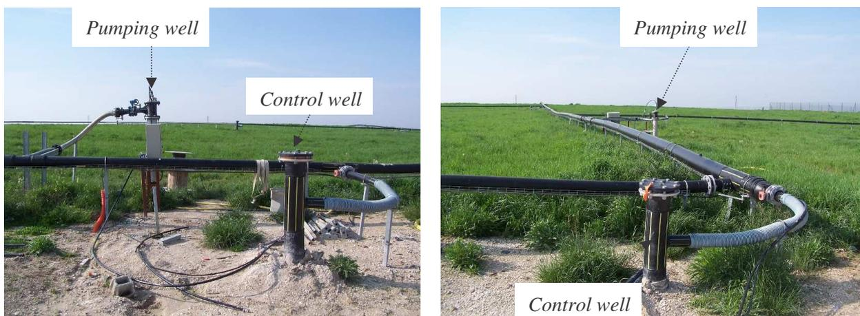
Figure 1. Associated pumping and control wells on the experimental cell.
