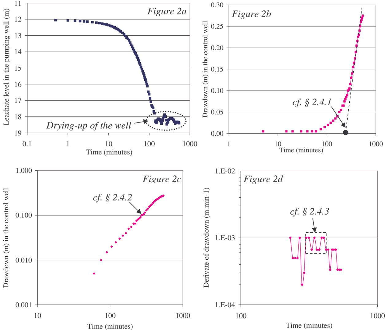
Figure 2. Experimental results from pumping tests (2a: pumping well; 2b/c/d: control wells).
