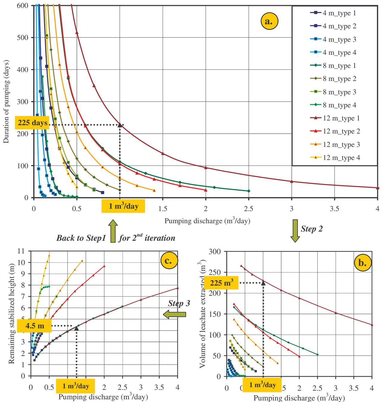
Figure 4. Example of abacuses developed using Modflow-Surfact (Study case: width = 50 m \* 50 m; pumping well centered at the middle of the domain; initial level of saturation: 4, 8 or 12 m; other parameters: waste height + type of waste: unpublished).
