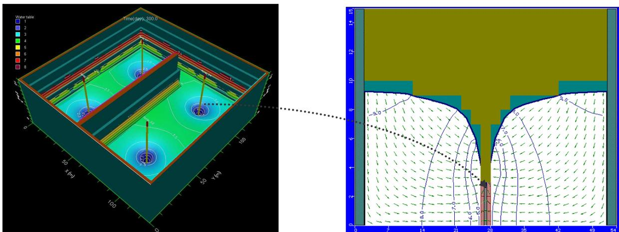
Figure 3. (a) Modeling the evolution of the leachate head using Visual Modflow 3D (Modflow-Surfact flow model). (b) Flow directions (arrows) and hydraulic equipotential lines during a pumping exercise.
